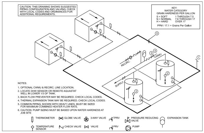
Figure 12. Water Heater Piping — Multiple Heaters, Multiple Tanks.
